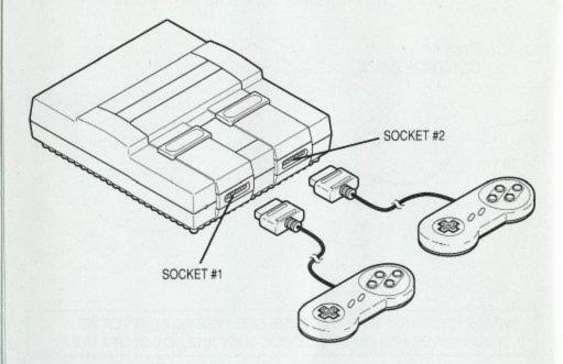
The two (2) Super NES Controllers are identical and can be plugged into either socket number, but the *select* and *start* buttons will work only on the controller plugged into socket #1. For one-player games or when you are playing a game alone, the controller must be plugged into socket #1.
