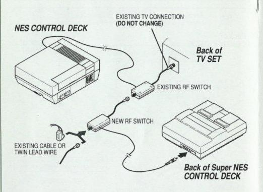
NOTE: This method of connection will produce mono sound only (the left and right stereo channels are mixed).
