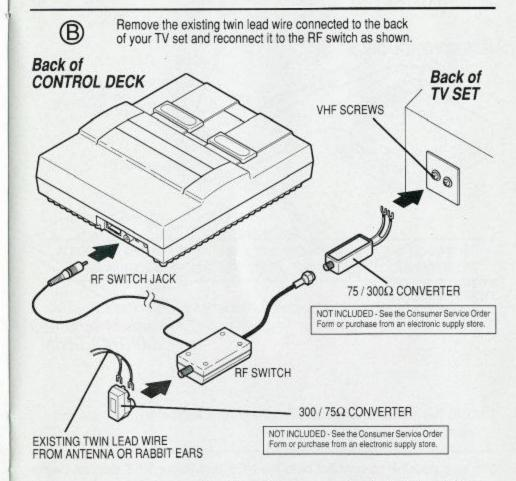
NOTE: This method of connection will produce mono sound only (the left and right stereo channels are mixed).
