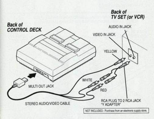
NOTE: This method of connection will produce mono sound only (the left and right stereo channels are mixed).
