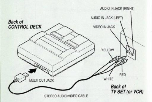
NOTE: This is the only method of connecting the Super NES Control Deck to a TV to get the full effects of the stereo sound. It is also possible to connect the audio output of the Control Deck to a stereo system. For additional information on this type of connection call: 1-800-255-3700
