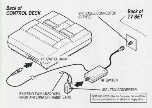
NOTE: This method of connection will produce mono sound only (the left and right stereo channels are mixed).
